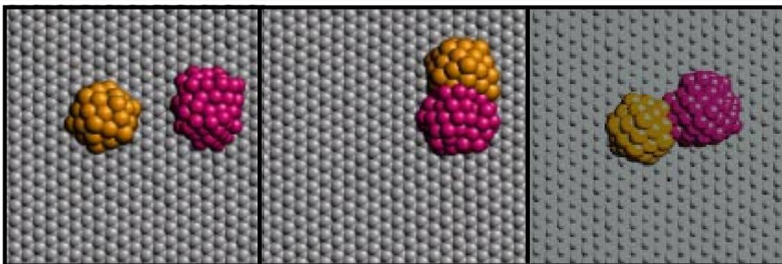
Fig. 3.2.4: Thermally activated diffusion and sintering of Pt nanoclusters on (111) diamond. Shown are snapshots after 15ps, 45ps and 250 ps.
