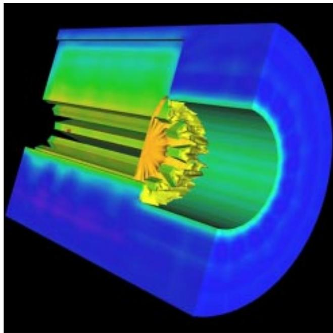
Fig. 3.2.2: Propellant average stress and gas pressure in fully 3-D, integrated GEN1 simulation.
