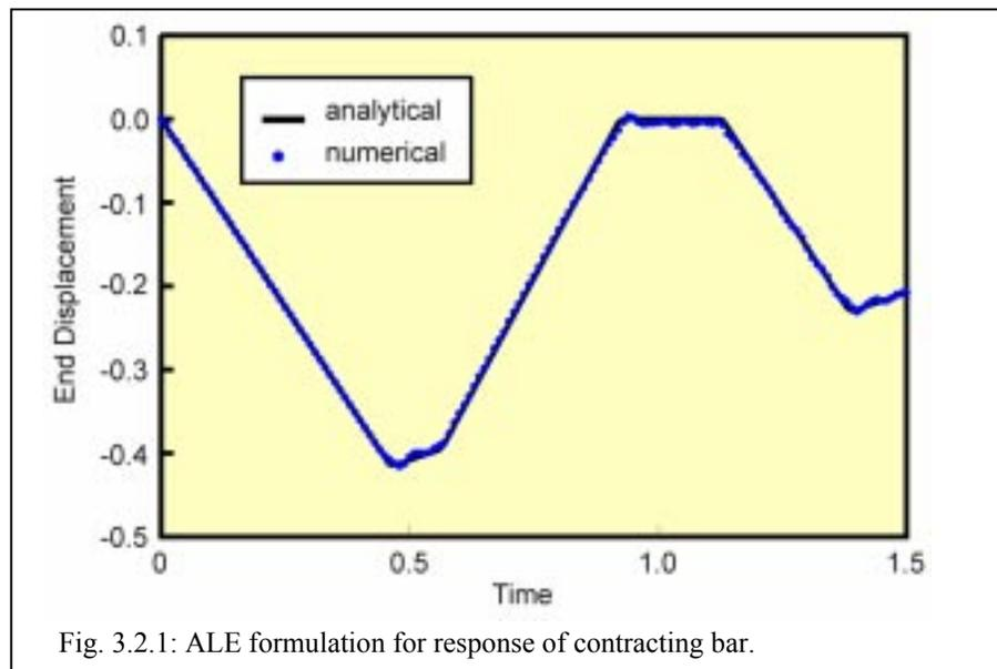
Fig. 3.2.1: ALE formulation for response of contracting bar.
