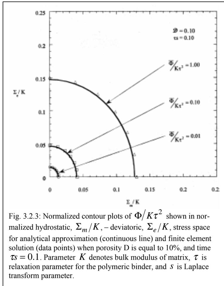
Fig. 3.2.3: Normalized contour plots of  $\Phi / K\tau^2$  shown in normalized hydrostatic,  $\Sigma_m / K$ , – deviatoric,  $\Sigma_e / K$ , stress space for analytical approximation (continuous line) and finite element solution (data points) when porosity  $D$  is equal to 10%, and time  $\tau s = 0.1$ . Parameter  $K$  denotes bulk modulus of matrix,  $\tau$  is relaxation parameter for the polymeric binder, and  $s$  is Laplace transform parameter.
