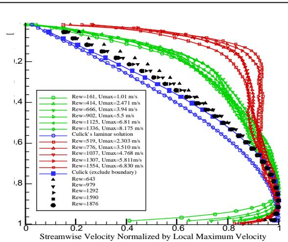
Fig. 3.3.6: Streamwise velocity profiles from planar rocket chamber simulation experiment.
