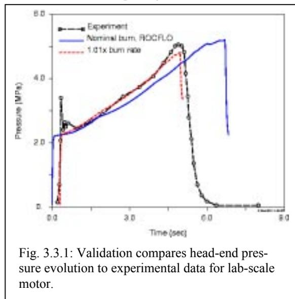
Fig. 3.3.1: Validation compares head-end pressure evolution to experimental data for lab-scale motor.
