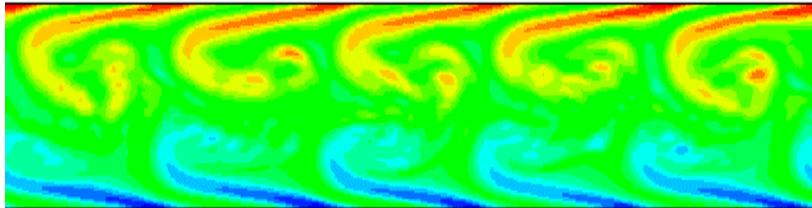
Fig. 3.3.4: Spanwise vorticity in compressible periodic rocket simulation.
