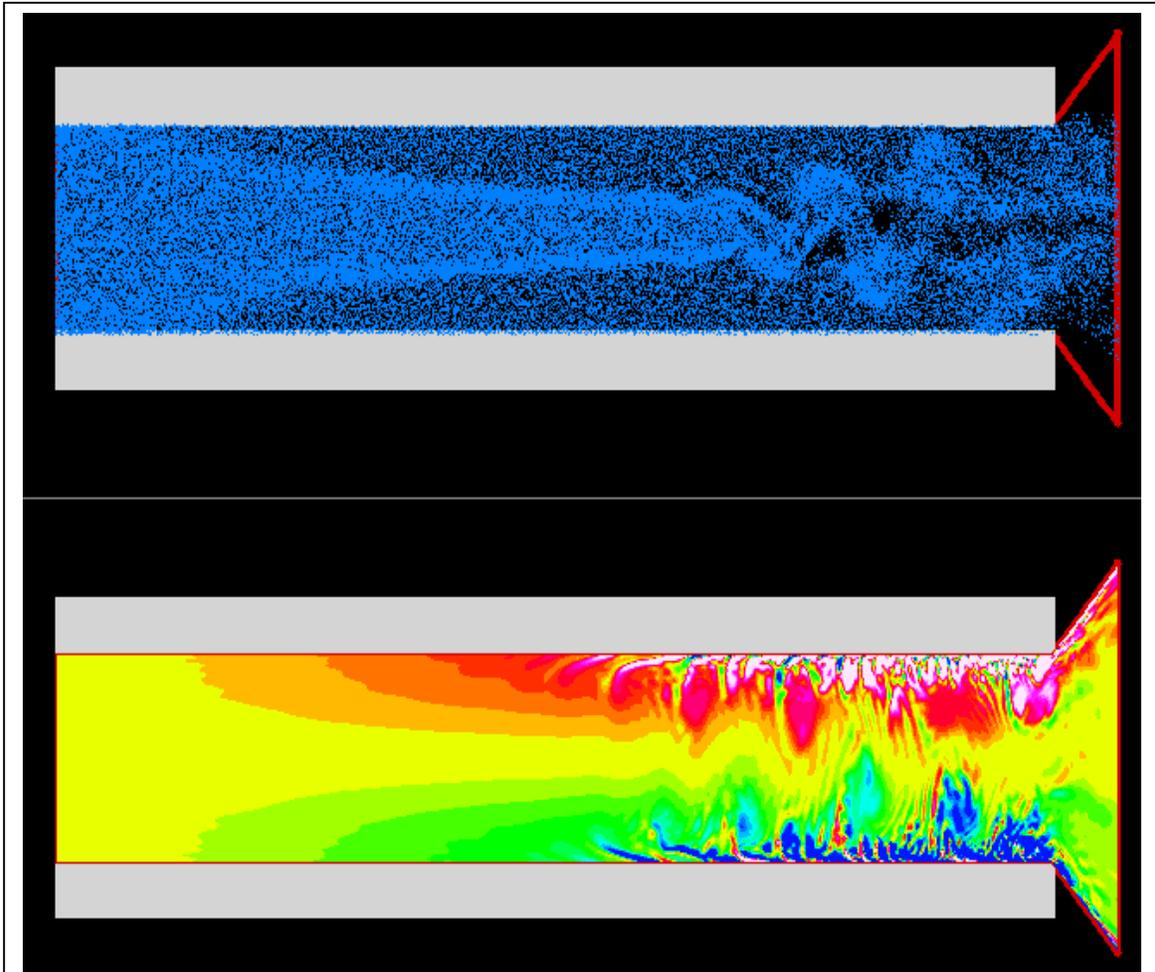
Fig. 3.3.3: Distribution of aluminum droplets in simulated core flow. Top image shows 90000 droplets tracked in computational domain. Bottom image shows spanwise vorticity. White/red represent positive vorticity, blue/green is negative.
