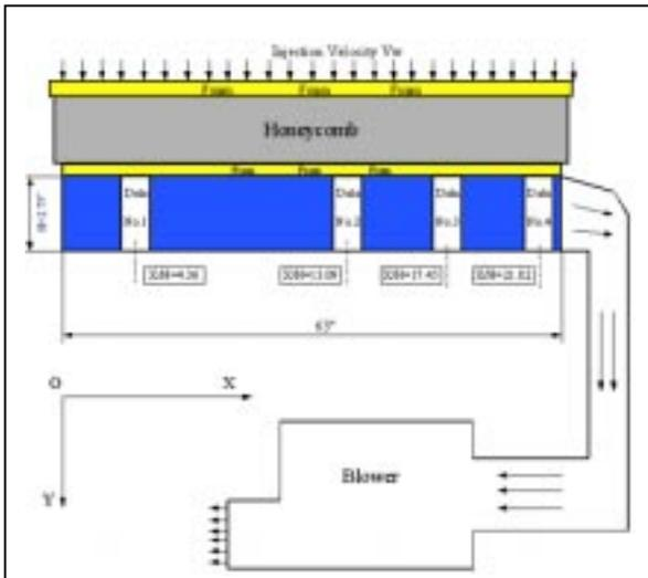
Fig. 3.3.5: Schematic of planar rocket chamber simulation experiment.
