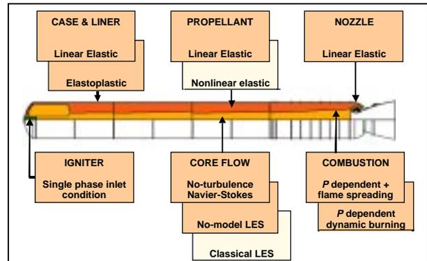
Fig. 2.3: GEN1 Simulation Roadmap provides direction for future research. Shaded boxes show completed tasks.
