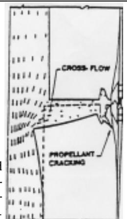
Fig. 2.8: PQM-1 failed due to excessive pressure drop and grain deformation near aft slot.
