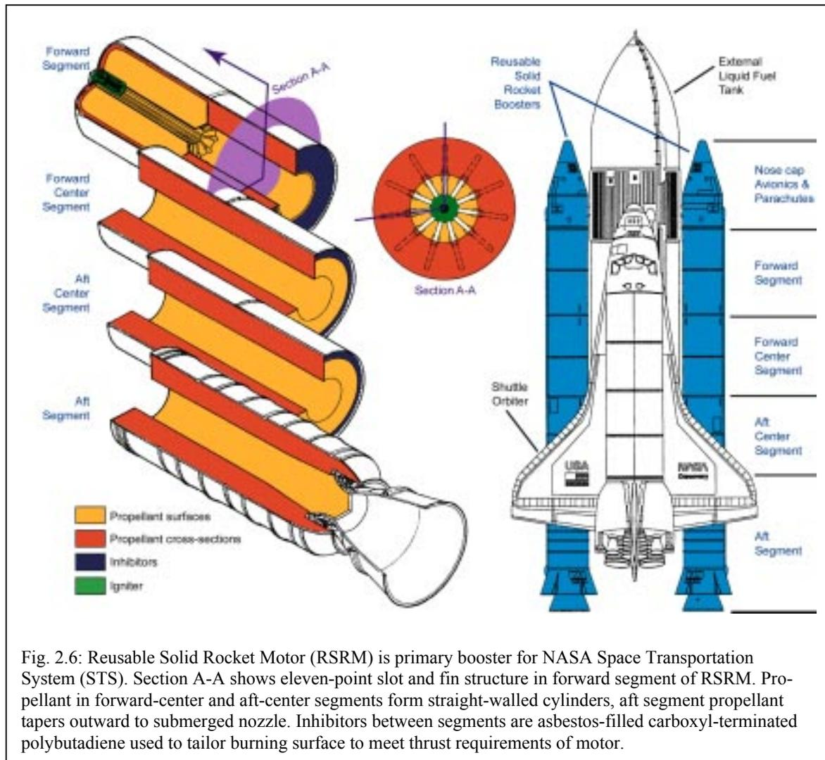
Fig. 2.6: Reusable Solid Rocket Motor (RSRM) is primary booster for NASA Space Transportation System (STS). Section A-A shows eleven-point slot and fin structure in forward segment of RSRM. Propellant in forward-center and aft-center segments form straight-walled cylinders, aft segment propellant tapers outward to submerged nozzle. Inhibitors between segments are asbestos-filled carboxyl-terminated polybutadiene used to tailor burning surface to meet thrust requirements of motor.
