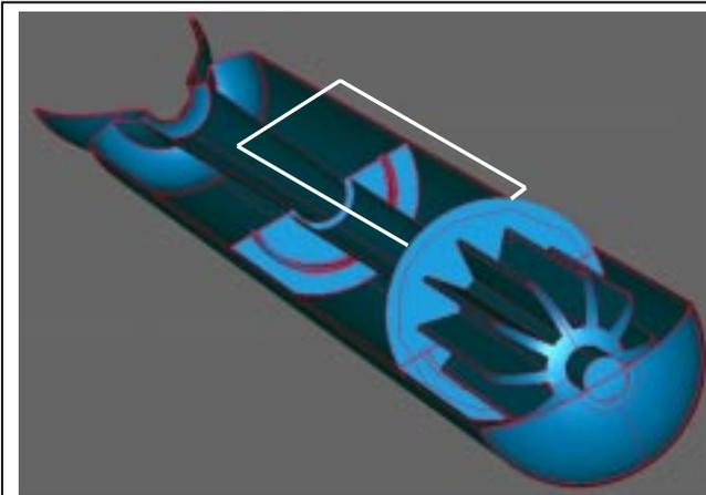
Fig. 2.7: Cutaway drawing of Titan IV PQM-1 motor shows three-segment solid propellant design.
