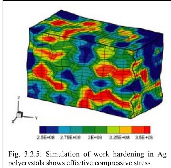
Fig. 3.2.5: Simulation of work hardening in Ag polycrystals shows effective compressive stress.
