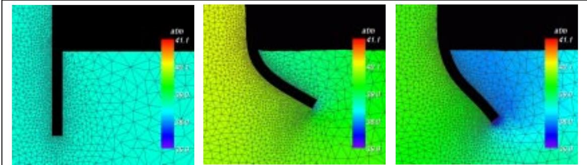
Fig. 3.2.1: Evolution of fluid mesh in vicinity of aeroelastically deforming inhibitor at times  $t = 0$  s. (left),  $t = 0.024$  s. (center) and  $t = 0.036$  s. (right). Sequence demonstrates mesh repair capabilities present in fluid solver and large deformations experienced by flexible inhibitor. Color contours denote pressure.
