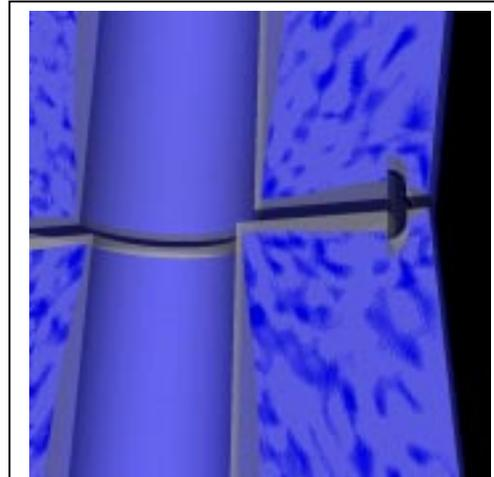
Fig. 3.2.2: *Rocfrac* is used to simulate Titan IV slumping failure. Undeformed (gray) and deformed (blue) solid at  $t = 10$  ms,  $P = 100$  MPa.
