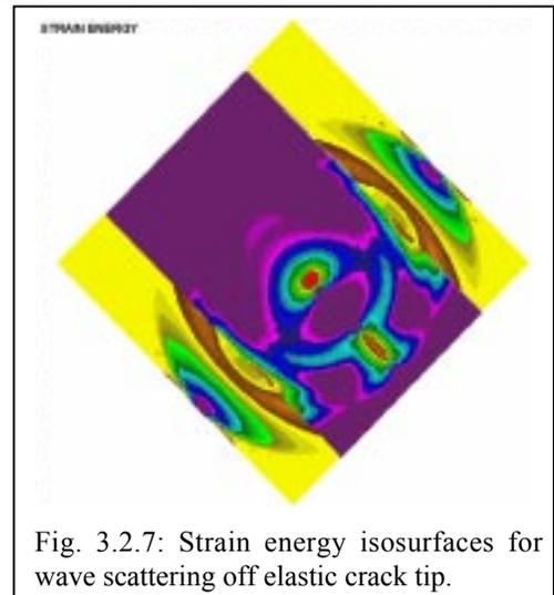
Fig. 3.2.7: Strain energy isosurfaces for wave scattering off elastic crack tip.
