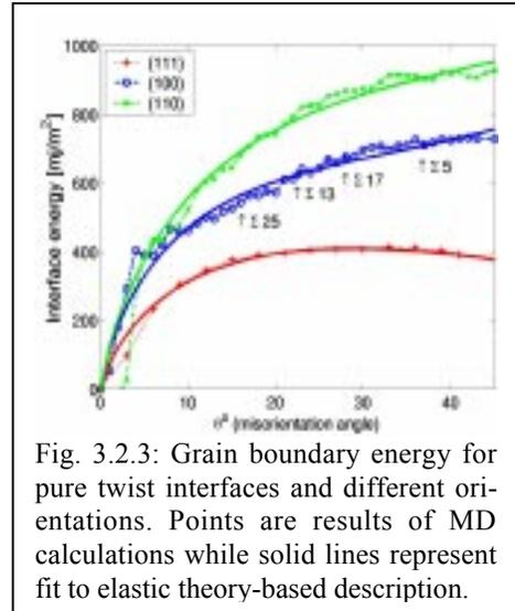
Fig. 3.2.3: Grain boundary angle energy for pure twist interfaces and different orientations. Points are results of MD calculations while solid lines represent fit to elastic theory-based description.
