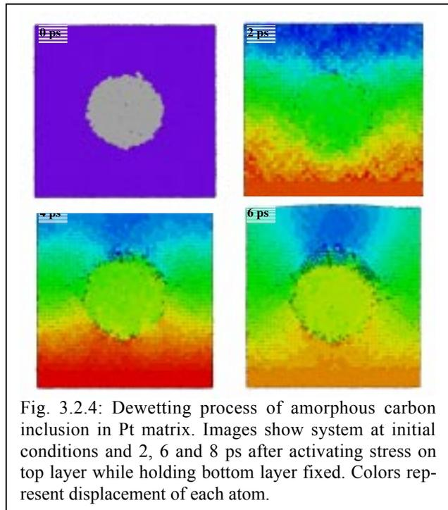
Fig. 3.2.4: Dewetting process of amorphous carbon inclusion in Pt matrix. Images show system at initial conditions and 2, 6 and 8 ps after activating stress on top layer while holding bottom layer fixed. Colors represent displacement of each atom.
