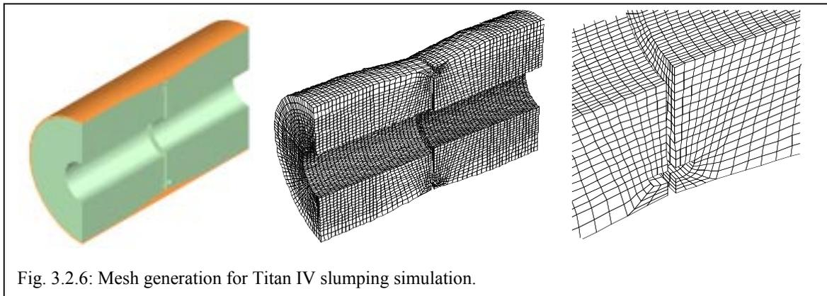
Fig. 3.2.6: Mesh generation for Titan IV slumping simulation.
