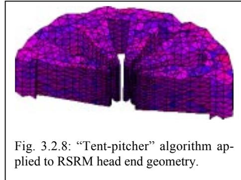
Fig. 3.2.8: "Tent-pitcher" algorithm applied to RSRM head end geometry.
