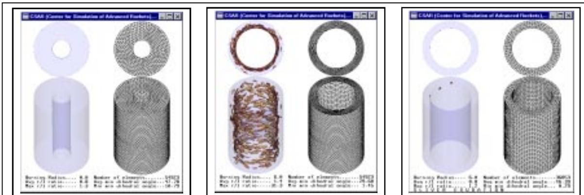
Fig. 3.4.5: Mesh repair is critical to solid rocket combustion simulations. Shown here are initial mesh prior to any combustion, “bad” elements and mesh after 60% of propellant has burned away, and repaired mesh.
