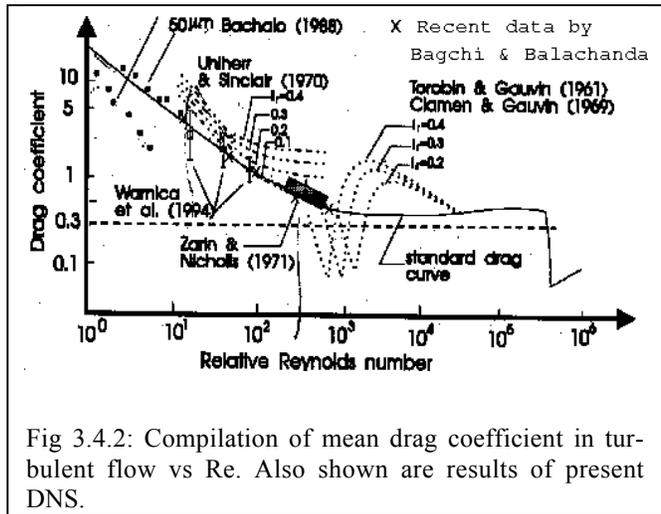
Fig 3.4.2: Compilation of mean drag coefficient in turbulent flow vs Re. Also shown are results of present DNS.
