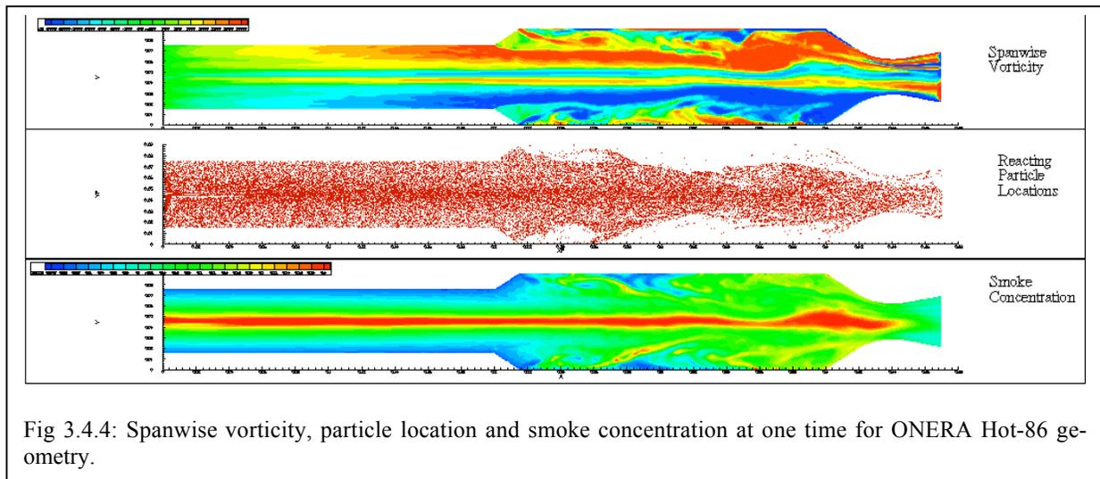
Fig 3.4.4: Spanwise vorticity, particle location and smoke concentration at one time for ONERA Hot-86 geometry.
