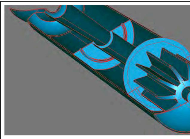
Fig. 2.5: Cutaway drawing of Titan IV PQM-1 motor shows three-segment solid propellant design.
