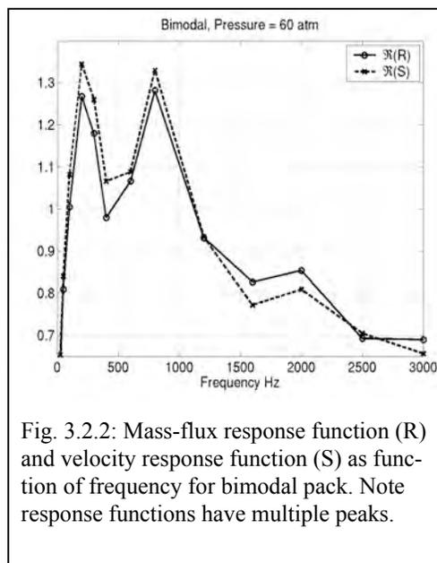
Fig. 3.2.2: Mass-flux response function (R) and velocity response function (S) as function of frequency for bimodal pack. Note response functions have multiple peaks.
