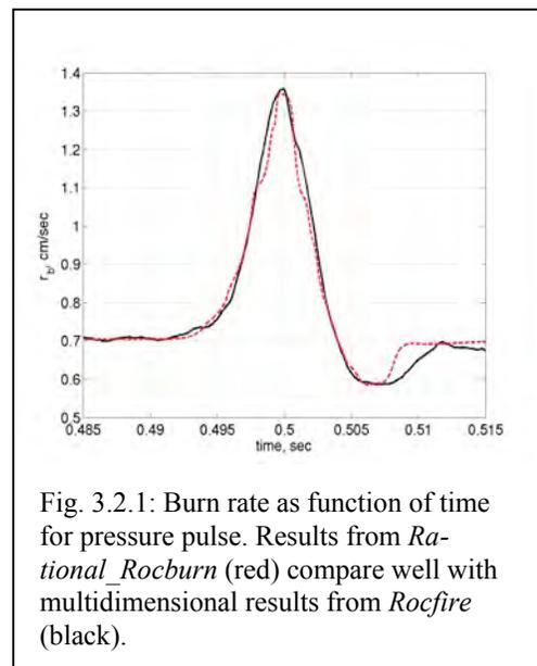
Fig. 3.2.1: Burn rate as function of time for pressure pulse. Results from *Rational Rocburn* (red) compare well with multidimensional results from *Rocfire* (black).
