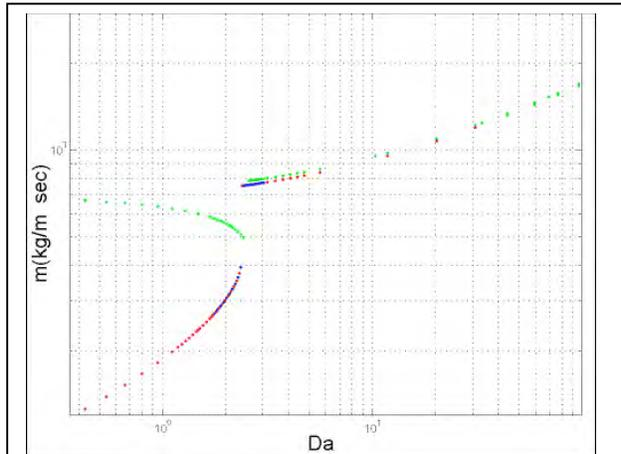
Fig. 3.2.11: Quasi-steady calculation of mass flux for small Damkohler numbers
