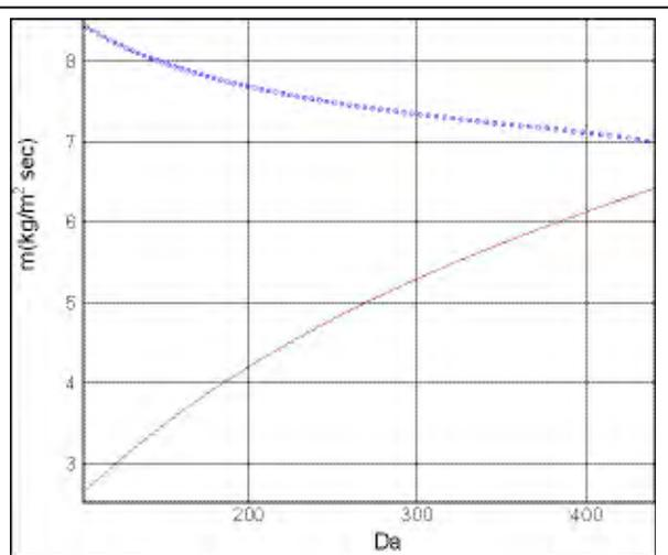
Fig. 3.2.10: Results of two experiments of burning 0.001 m diameter HMX particle with varying Damkohler number, which is proportional to product of particle radius and ambient pressure squared, by decreasing ambient pressure from 20atm and keeping radius of particle constant (blue curve), and by decreasing radius of particle and keeping pressure con-
