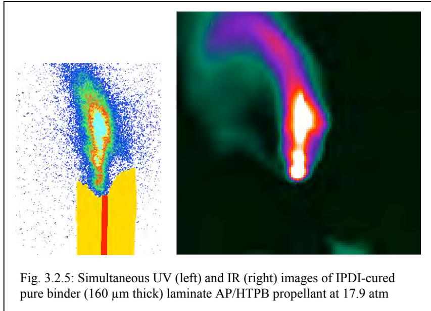
Fig. 3.2.5: Simultaneous UV (left) and IR (right) images of IPDI-cured pure binder (160  $\mu\text{m}$  thick) laminate AP/HTPB propellant at 17.9 atm
