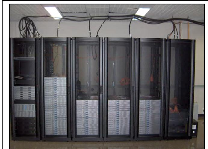
Fig. 3.3.5: Initial 64 nodes of new Apple G5 cluster. Complete cluster is 640 dual-processor nodes (1280 processors).
