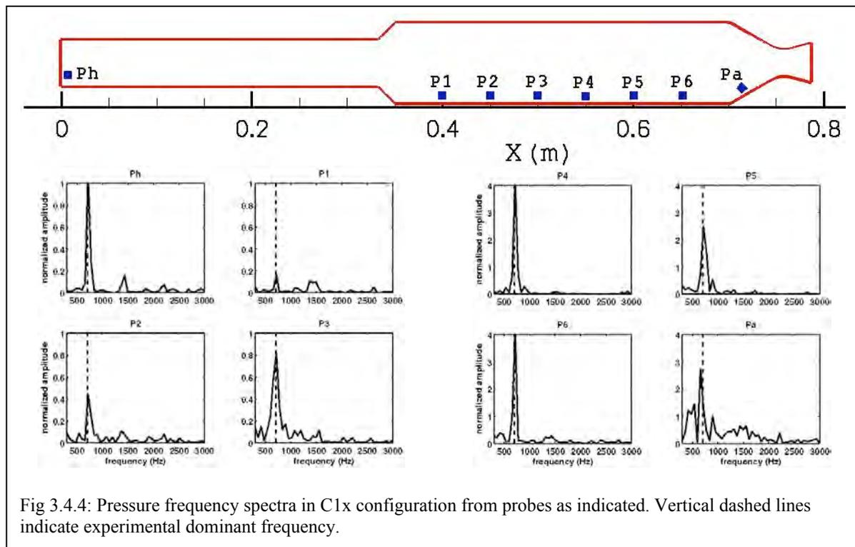
Fig 3.4.4: Pressure frequency spectra in C1x configuration from probes as indicated. Vertical dashed lines indicate experimental dominant frequency.
