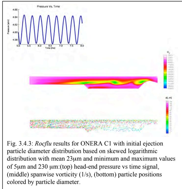
Fig. 3.4.3: *Rocflu* results for ONERA C1 with initial ejection particle diameter distribution based on skewed logarithmic distribution with mean  $23\mu\text{m}$  and minimum and maximum values of  $5\mu\text{m}$  and  $230\mu\text{m}$ : (top) head-end pressure vs time signal, (middle) spanwise vorticity (1/s), (bottom) particle positions colored by particle diameter.
