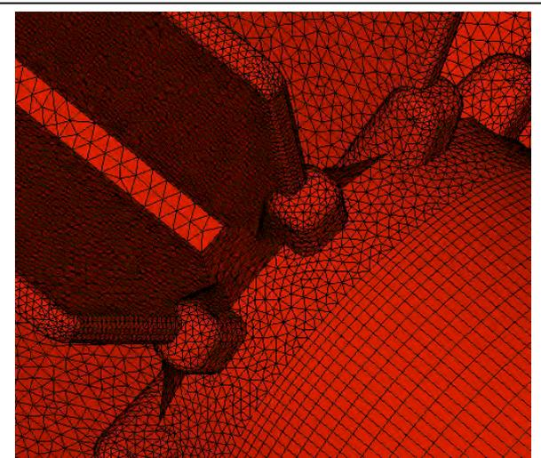
Fig. 3.4.1: *Rocflu* unstructured grid of RSRM star-grain stress relief notches
