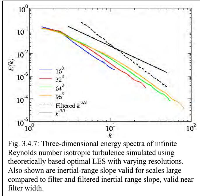
Fig. 3.4.7: Three-dimensional energy spectra of infinite Reynolds number isotropic turbulence simulated using theoretically based optimal LES with varying resolutions. Also shown are inertial-range slope valid for scales large compared to filter and filtered inertial range slope, valid near filter width.
