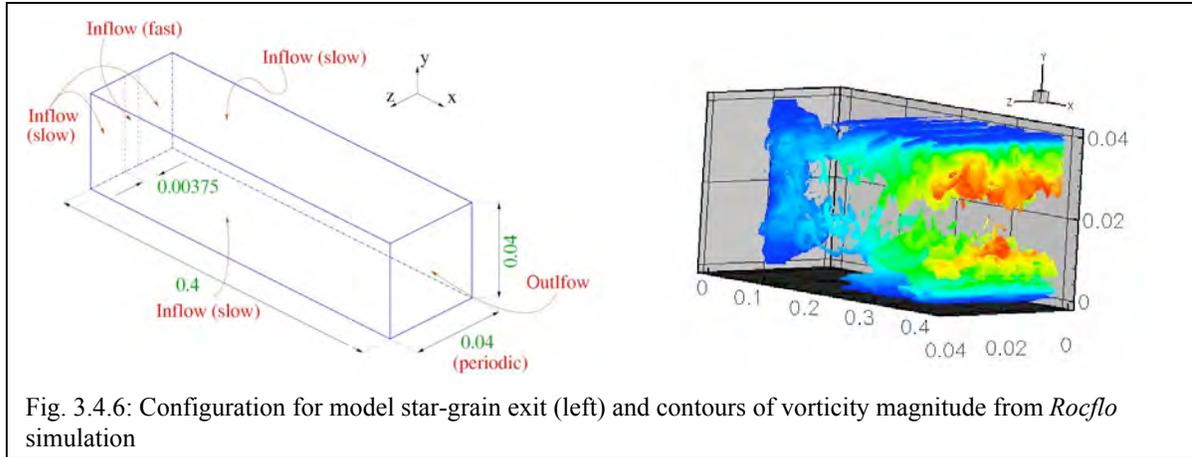
Fig. 3.4.6: Configuration for model star-grain exit (left) and contours of vorticity magnitude from *Rocflo* simulation
