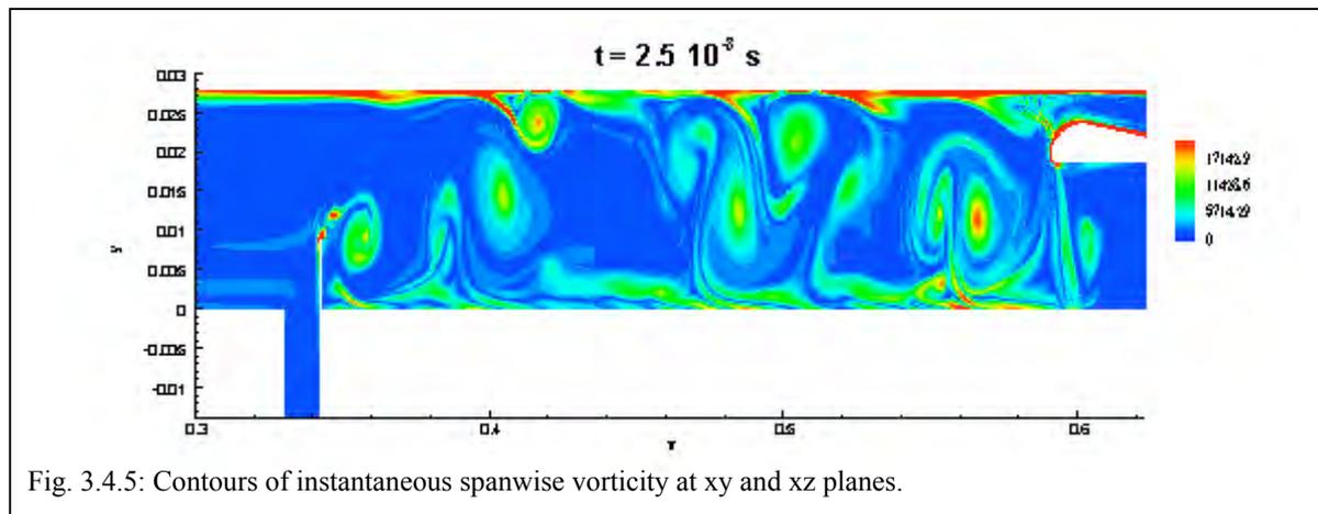
Fig. 3.4.5: Contours of instantaneous spanwise vorticity at xy and xz planes.
