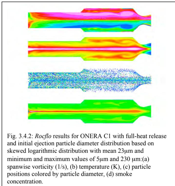
Fig. 3.4.2: *Rocflo* results for ONERA C1 with full-heat release and initial ejection particle diameter distribution based on skewed logarithmic distribution with mean  $23\mu\text{m}$  and minimum and maximum values of  $5\mu\text{m}$  and  $230\mu\text{m}$ :(a) spanwise vorticity (1/s), (b) temperature (K), (c) particle positions colored by particle diameter, (d) smoke concentration.
