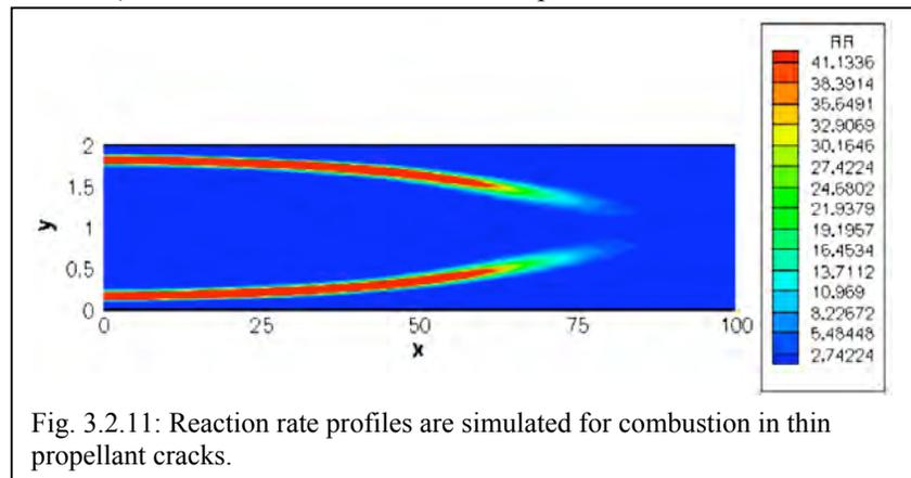
Fig. 3.2.11: Reaction rate profiles are simulated for combustion in thin propellant cracks.
