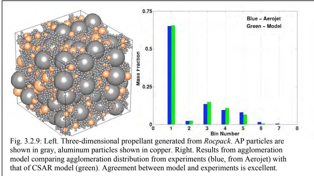
Fig. 3.2.9: Left. Three-dimensional propellant generated from *Rocpack*. AP particles are shown in gray, aluminum particles shown in copper. Right. Results from agglomeration model comparing agglomeration distribution from experiments (blue, from Aerojet) with that of CSAR model (green). Agreement between model and experiments is excellent.
