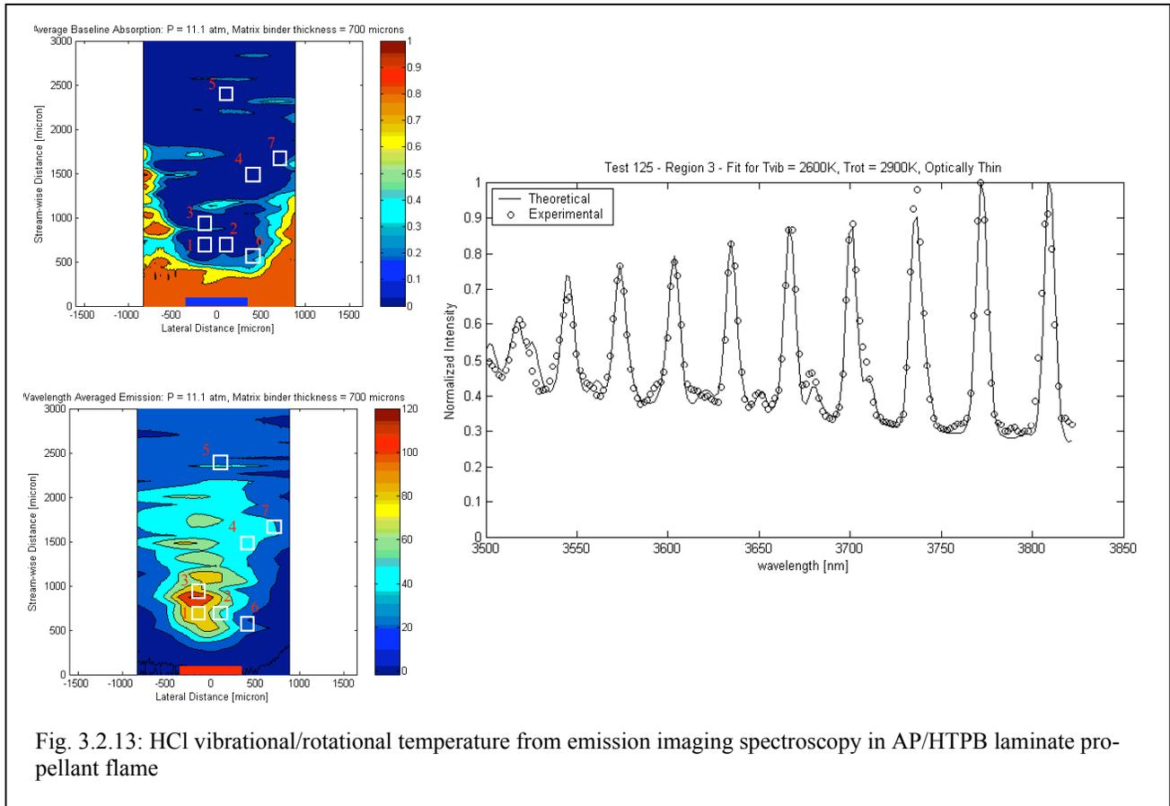
Fig. 3.2.13: HCl vibrational/rotational temperature from emission imaging spectroscopy in AP/HTPB laminate propellant flame
