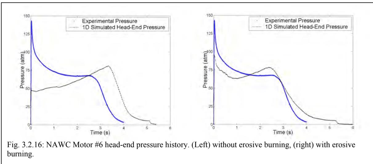
Fig. 3.2.16: NAWC Motor #6 head-end pressure history. (Left) without erosive burning, (right) with erosive burning.
