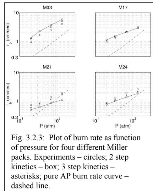
Fig. 3.2.3: Plot of burn rate as function of pressure for four different Miller packs. Experiments – circles; 2 step kinetics – box; 3 step kinetics – asterisks; pure AP burn rate curve – dashed line.
