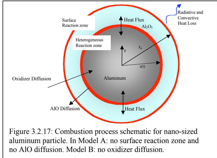
Figure 3.2.17: Combustion process schematic for nano-sized aluminum particle. In Model A: no surface reaction zone and no AIO diffusion. Model B: no oxidizer diffusion.
