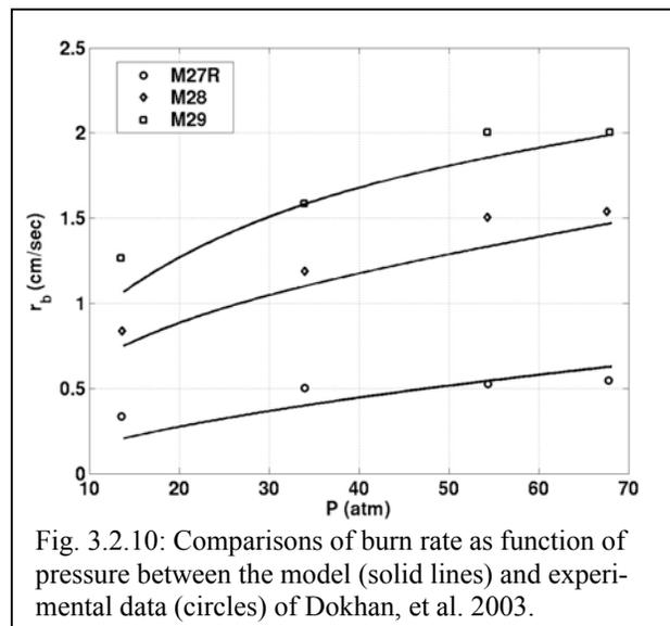
Fig. 3.2.10: Comparisons of burn rate as function of pressure between the model (solid lines) and experimental data (circles) of Dokhan, et al. 2003.
