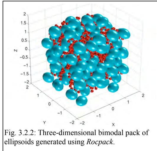
Fig. 3.2.2: Three-dimensional bimodal pack of ellipsoids generated using *Rocpack*.
