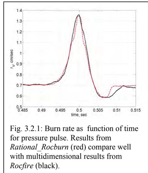
Fig. 3.2.1: Burn rate as function of time for pressure pulse. Results from *Rational Rocburn* (red) compare well with multidimensional results from *Rocfire* (black).
