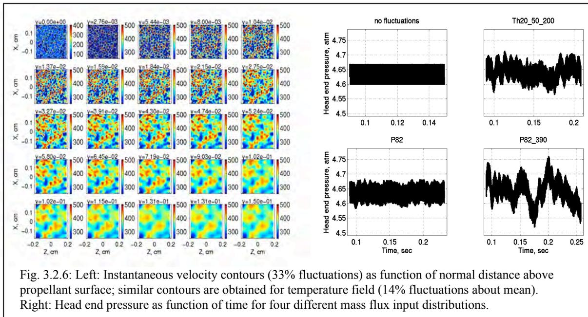
Fig. 3.2.6: Left: Instantaneous velocity contours (33% fluctuations) as function of normal distance above propellant surface; similar contours are obtained for temperature field (14% fluctuations about mean). Right: Head end pressure as function of time for four different mass flux input distributions.
