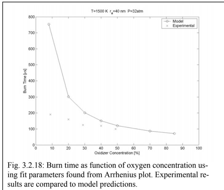
Fig. 3.2.18: Burn time as function of oxygen concentration using fit parameters found from Arrhenius plot. Experimental results are compared to model predictions.
