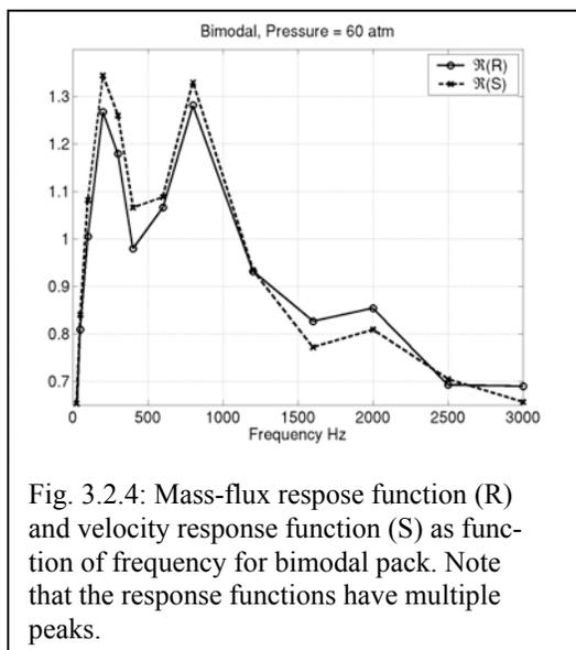
Fig. 3.2.4: Mass-flux response function (R) and velocity response function (S) as function of frequency for bimodal pack. Note that the response functions have multiple peaks.
