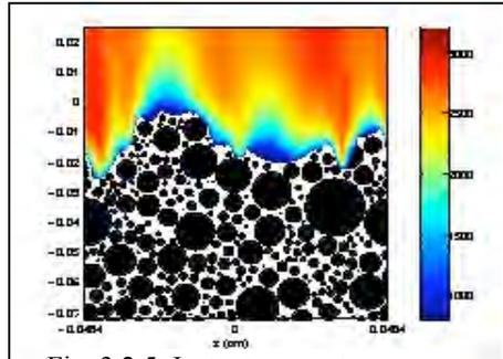
Fig. 3.2.5: Instantaneous temperature contours for HMX/HTPB propellant; slice through three-dimensional pack.
