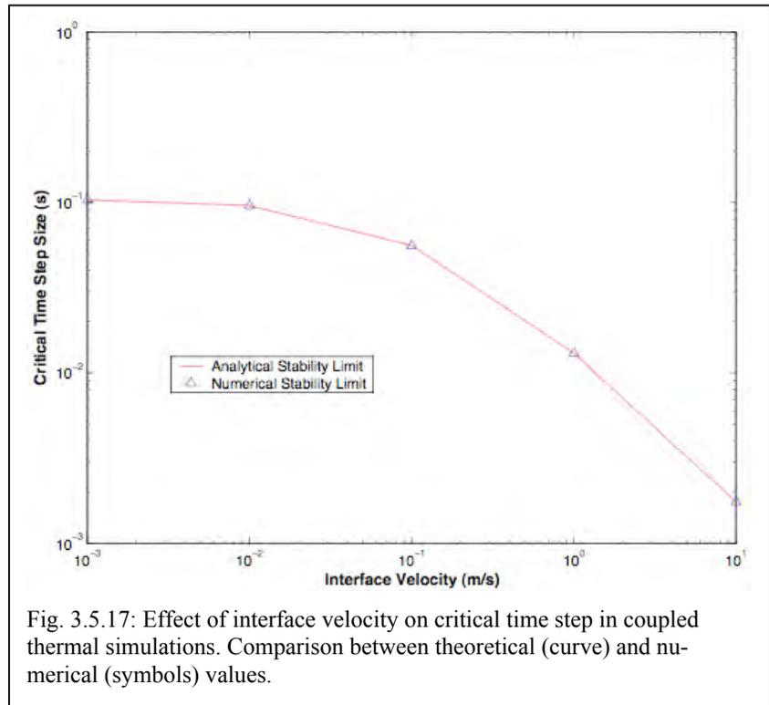
Fig. 3.5.17: Effect of interface velocity on critical time step in coupled thermal simulations. Comparison between theoretical (curve) and numerical (symbols) values.
