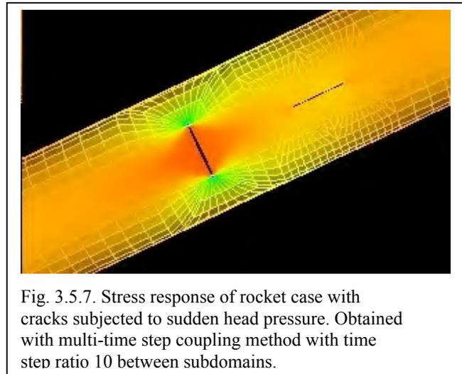
Fig. 3.5.7. Stress response of rocket case with cracks subjected to sudden head pressure. Obtained with multi-time step coupling method with time step ratio 10 between subdomains.
