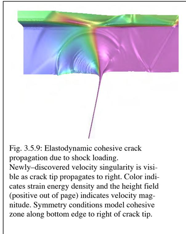
Fig. 3.5.9: Elastodynamic cohesive crack propagation due to shock loading. Newly-discovered velocity singularity is visible as crack tip propagates to right. Color indicates strain energy density and the height field (positive out of page) indicates velocity magnitude. Symmetry conditions model cohesive zone along bottom edge to right of crack tip.
