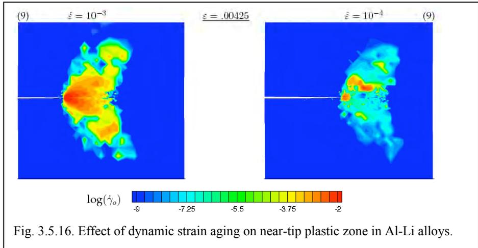
Fig. 3.5.16. Effect of dynamic strain aging on near-tip plastic zone in Al-Li alloys.
