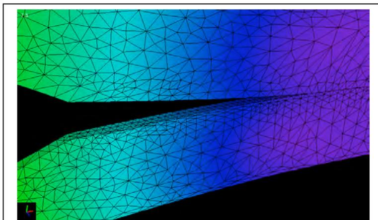
Fig. 3.5.1: Dynamic fracture of Double Cantilever Beam (DCB) specimen modeled with 3D non-matching cohesive finite elements.
