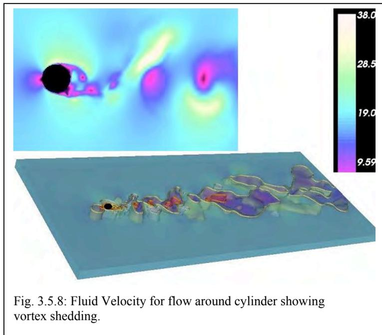
Fig. 3.5.8: Fluid Velocity for flow around cylinder showing vortex shedding.
