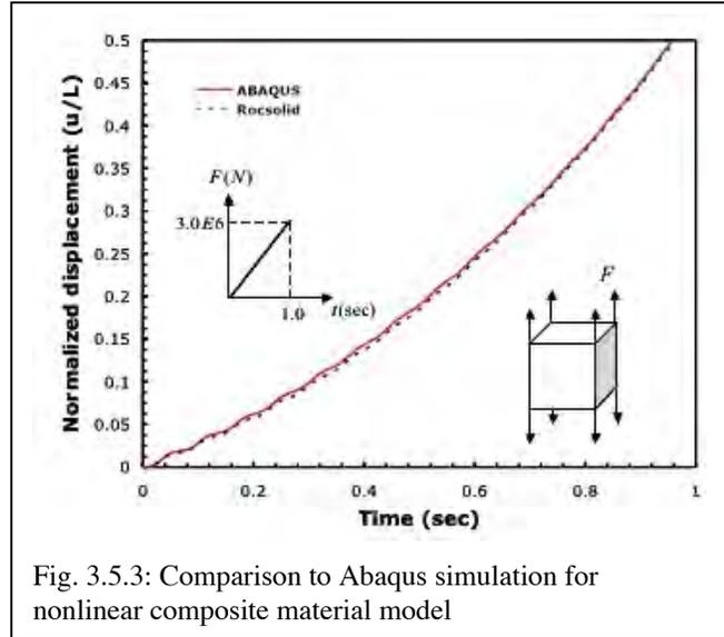
Fig. 3.5.3: Comparison to Abaqus simulation for nonlinear composite material model
