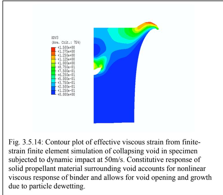
Fig. 3.5.14: Contour plot of effective viscous strain from finite-strain finite element simulation of collapsing void in specimen subjected to dynamic impact at 50m/s. Constitutive response of solid propellant material surrounding void accounts for nonlinear viscous response of binder and allows for void opening and growth due to particle dewetting.
