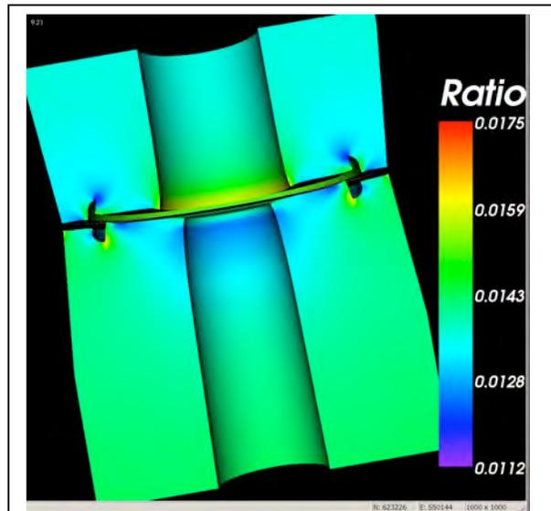
Fig. 3.5.4: Porosity distribution in propellant of Titan IV rocket motor near stress relief groove
