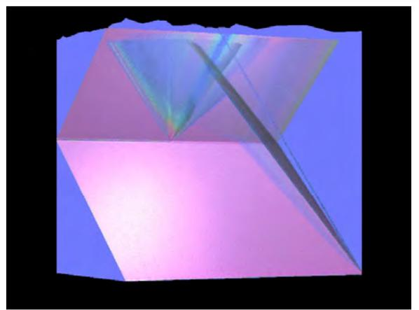
Fig. 3.5.10: Spacetime visualization of shock trajectories in crack-tip wave scattering. Vertical axis is time. (Visualization by Y. Zhou and M. Garland)
