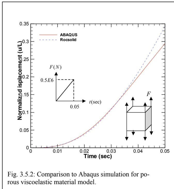
Fig. 3.5.2: Comparison to Abaqus simulation for porous viscoelastic material model.
