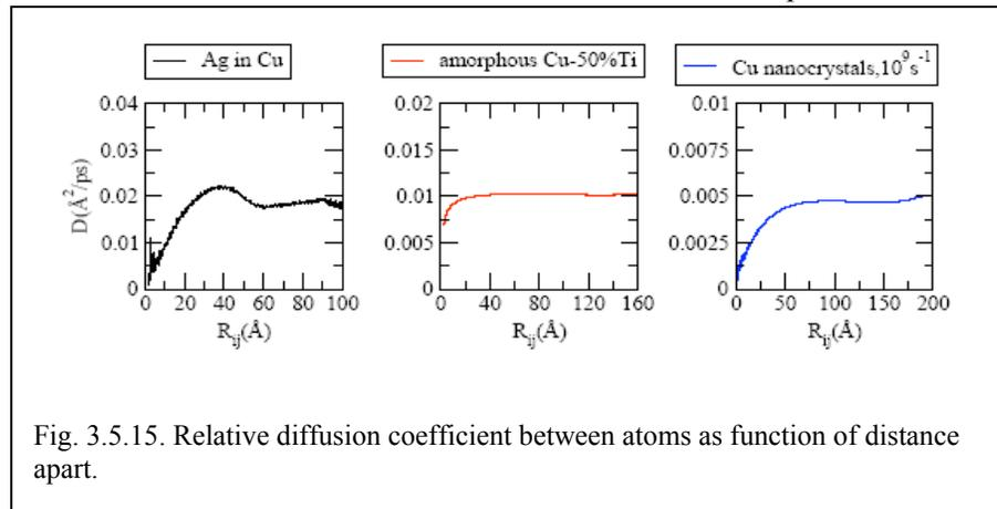
Fig. 3.5.15. Relative diffusion coefficient between atoms as function of distance apart.
