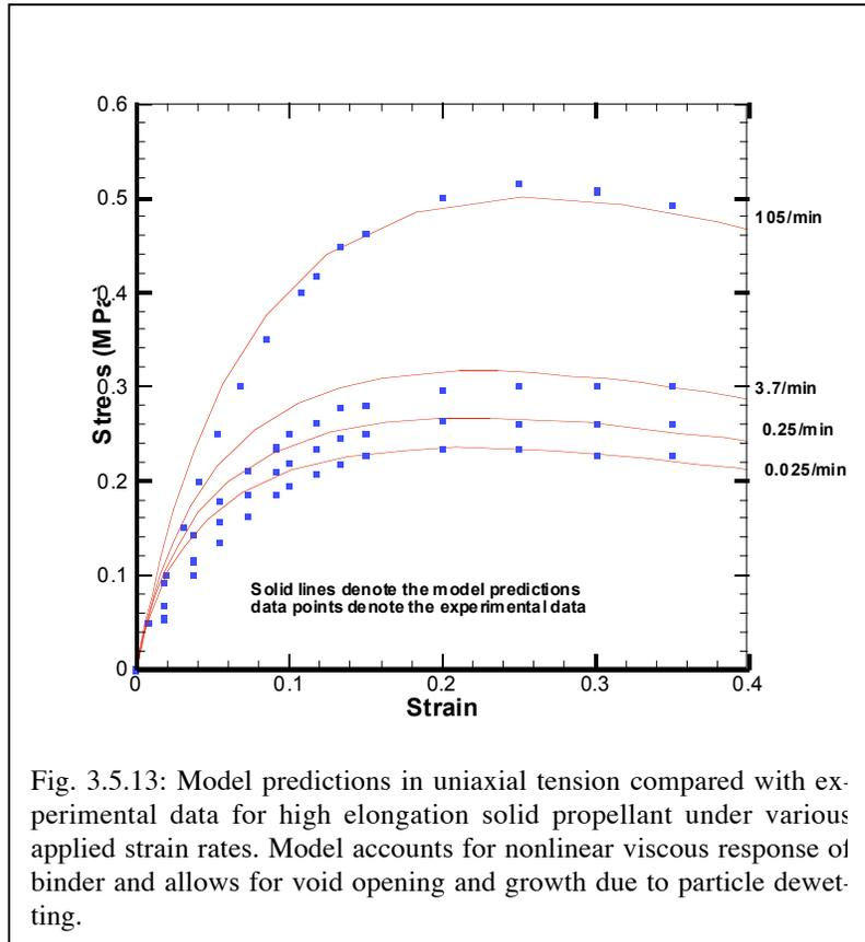
Fig. 3.5.13: Model predictions in uniaxial tension compared with experimental data for high elongation solid propellant under various applied strain rates. Model accounts for nonlinear viscous response of binder and allows for void opening and growth due to particle dewetting.
