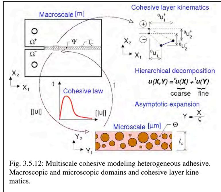
Fig. 3.5.12: Multiscale cohesive modeling heterogeneous adhesive. Macroscopic and microscopic domains and cohesive layer kinematics.
