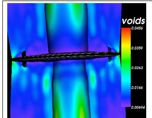
Fig. 3.5.5: Distribution of voids generated by dewetting of particles in Titan IV rocket motor grain
