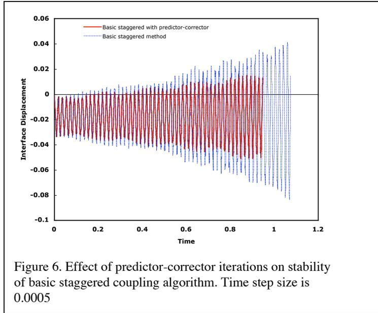
Figure 6. Effect of predictor-corrector iterations on stability of basic staggered coupling algorithm. Time step size is 0.0005
