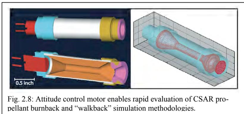
Fig. 2.8: Attitude control motor enables rapid evaluation of CSAR propellant burnback and “walkback” simulation methodologies.
