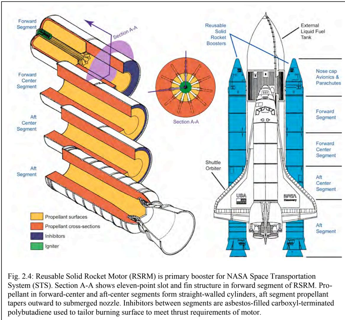
Fig. 2.4: Reusable Solid Rocket Motor (RSRM) is primary booster for NASA Space Transportation System (STS). Section A-A shows eleven-point slot and fin structure in forward segment of RSRM. Propellant in forward-center and aft-center segments form straight-walled cylinders, aft segment propellant tapers outward to submerged nozzle. Inhibitors between segments are asbestos-filled carboxyl-terminated polybutadiene used to tailor burning surface to meet thrust requirements of motor.
