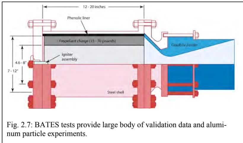
Fig. 2.7: BATES tests provide large body of validation data and aluminum particle experiments.
