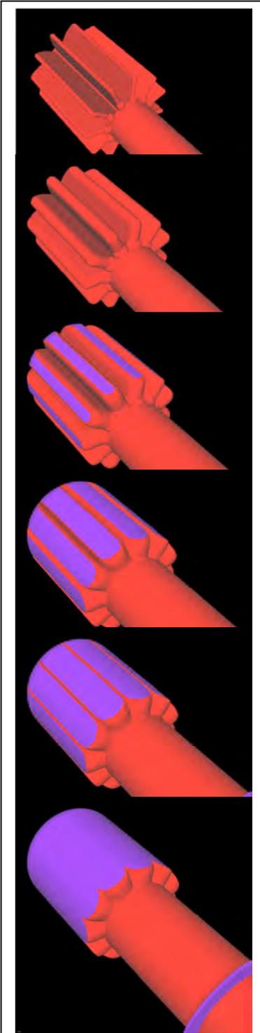
Fig 3.0.2: Complete propellant burnout in head end of RSRM (red is burning surface; blue is nonburning/extinguished).
