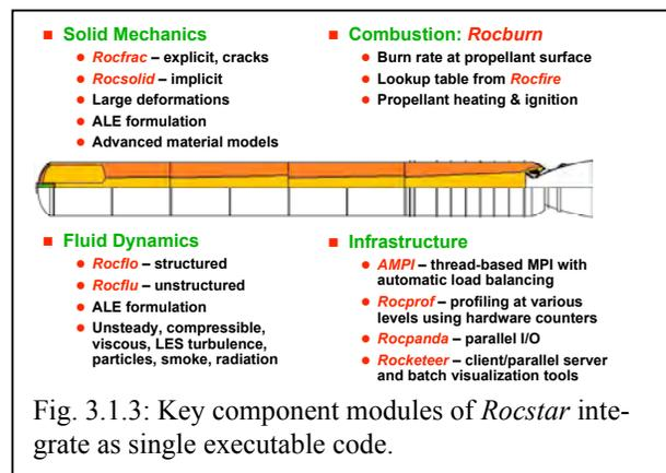
Fig. 3.1.3: Key component modules of *Rocstar* integrate as single executable code.
