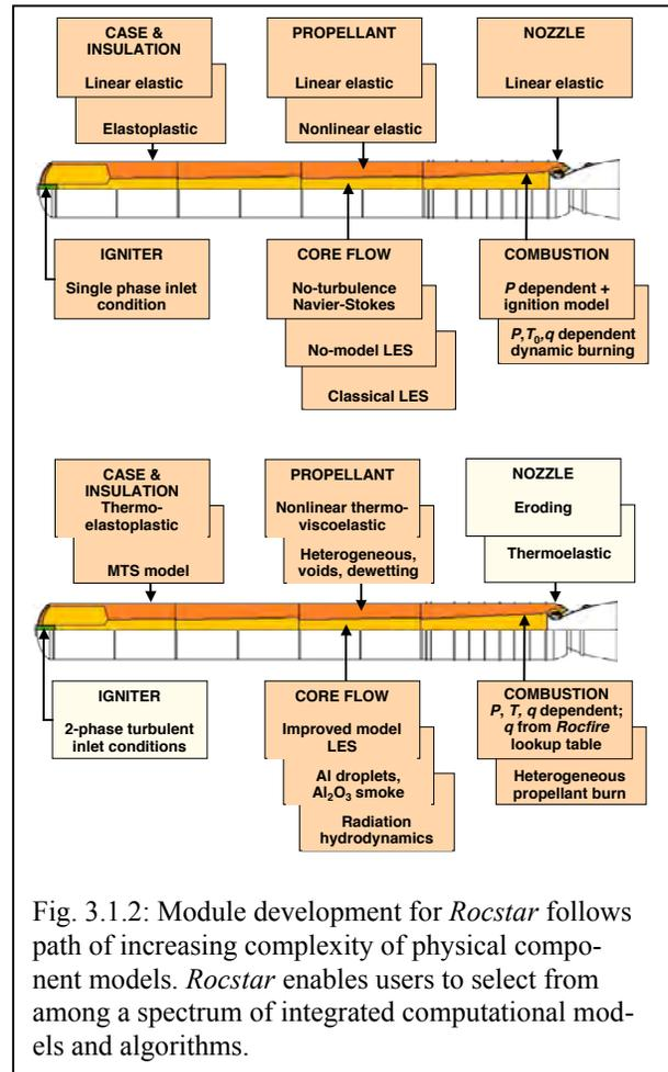
Fig. 3.1.2: Module development for *Rocstar* follows path of increasing complexity of physical component models. *Rocstar* enables users to select from among a spectrum of integrated computational models and algorithms.
