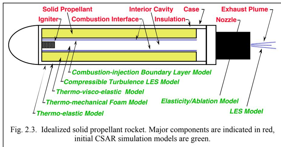
Fig. 2.3. Idealized solid propellant rocket. Major components are indicated in red, initial CSAR simulation models are green.
